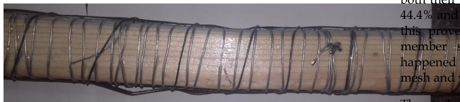
Failure in flexure: wood reference using Epoxy with thin wire
