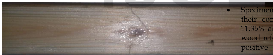
Failure in compression : wood reference with Epoxy
