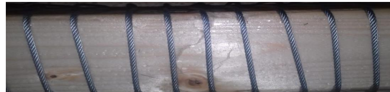
Failure in compression : wood reference using Epoxy with rolled wire
