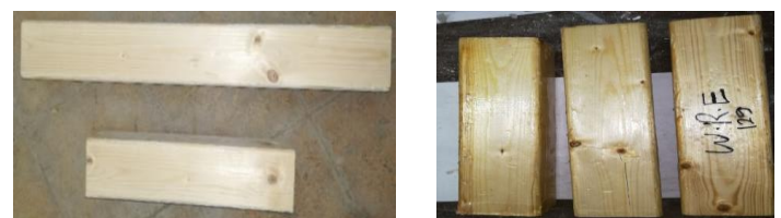
Fig. 4 (a): Compression and flexure samples, (b) : Samples with Epoxy 129
