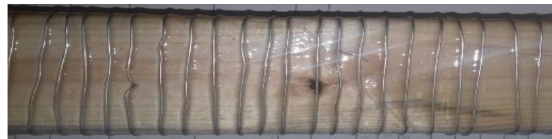
Failure in compression: wood reference using Epoxy with thin wire
